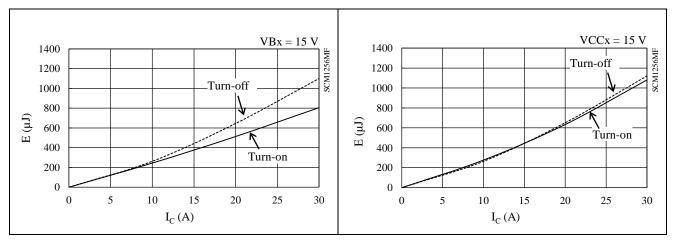
Figure 15-51. High-side Switching Loss ( $T_J = 25 \text{ °C}$ )
