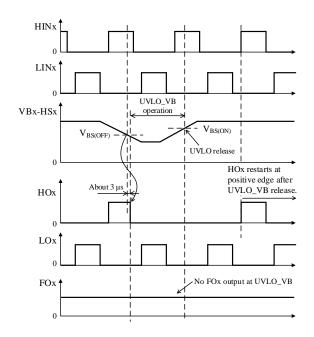
Figure 12-13. UVLO\_VB Operational Waveforms
