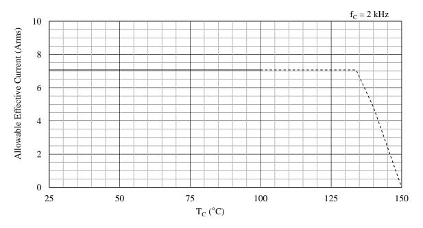
Figure 15-55. Allowable Effective Current ( $f_c = 2 \text{ kHz}$ ): 10 A Device
