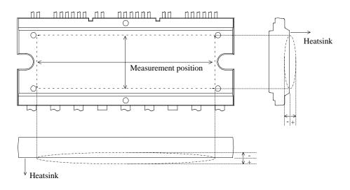
Figure 4-1. Flatness Measurement Position
