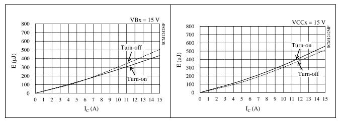
Figure 15-39 High-side Switching Loss ( $T_J = 25 \text{ °C}$ )
