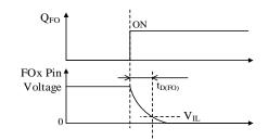
Figure 12-9. FOx Pin Delay Time, t<sub>D(FO)</sub>
