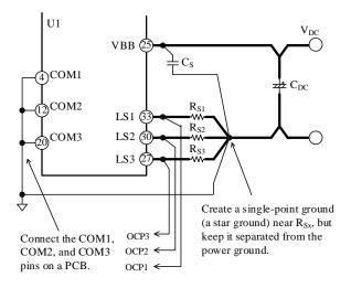
Figure 12-4. Connections to Logic Ground
