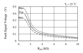
Figure 12-10. Fault Signal Voltage vs. Pull-up Resistor, R<sub>FO</sub>
