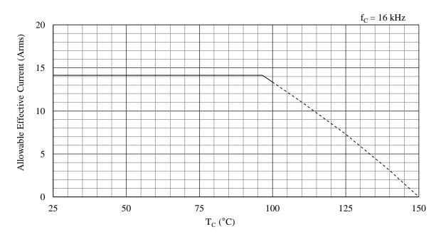
Figure 15-60. Allowable Effective Current ( $f_C = 16$  kHz): 20 A Devices
