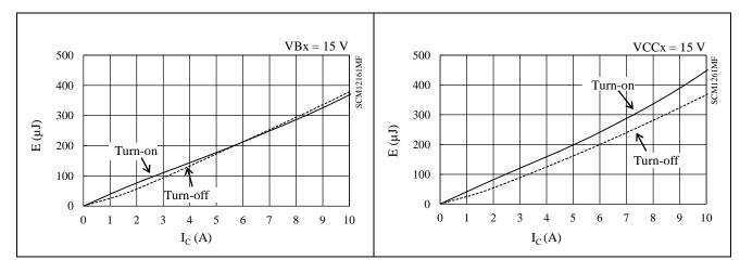
Figure 15-37. High-side Switching Loss ( $T_J = 125 \text{ °C}$ )
