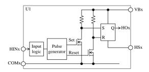
Figure 12-2. Internal Level-shifting Circuit
