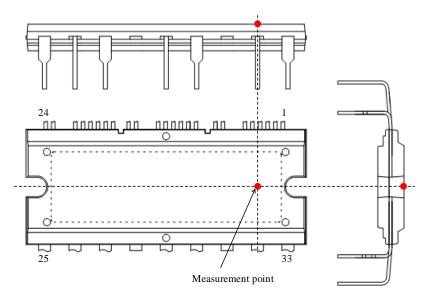
Figure 3-1. Case Temperature Measurement Point
