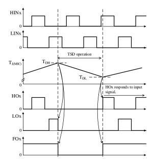
Figure 12-18. TSD Operational Waveforms
