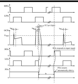
Figure 12-16. OCP Operational Waveforms
