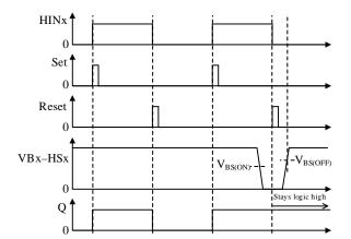
Figure 12-3. Waveforms at VBx-HSx Voltage Drop
