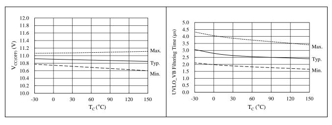
Figure 15-9. Logic Operation Stop Voltage,  $V_{CC(OFF)}$  vs.  $T_C$
