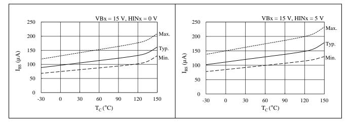
Figure 15-3. Logic Supply Current in 1-phase Operation (HINx = 0 V),  $I_{BS}$  vs.  $T_C$
