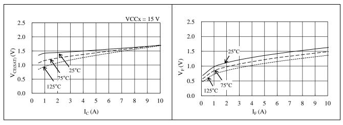
Figure 15-27. IGBT V<sub>CE(SAT)</sub> vs. I<sub>C</sub>
