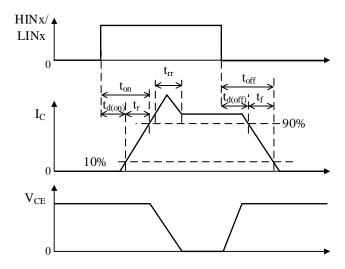
Figure 3-2. Switching Characteristics Definitions
