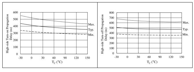
Figure 15-15. High-side Turn-on Propagation Delay vs.  $T_C$  (from HINx to HOx)
