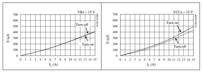
Figure 15-43 High-side Switching Loss ( $T_J = 25 \text{ °C}$ )
