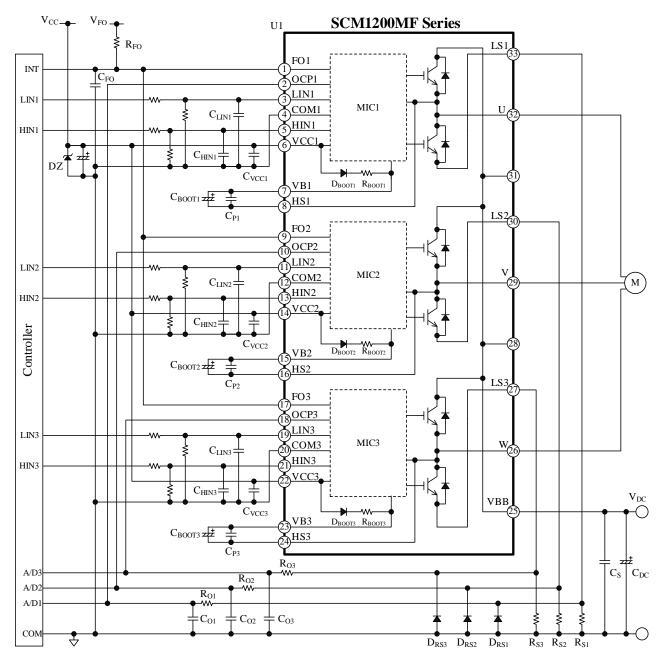
Figure 9-1. Typical Application Using Three Shunt Resistors
