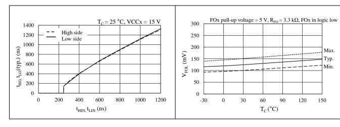
Figure 15-21. Typical Output Pulse Widths,  $t_{HO,}\,t_{LO}$  vs. Input Pulse Widths,  $t_{HIN,}\,t_{LIN}$
