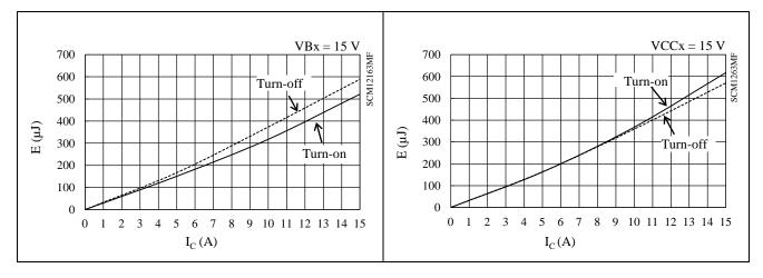
Figure 15-45. High-side Switching Loss ( $T_J = 125 \ ^{\circ}C$ )
