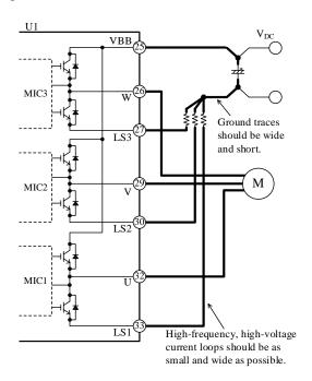
Figure 13-1. High-frequency, High-voltage Current Paths
