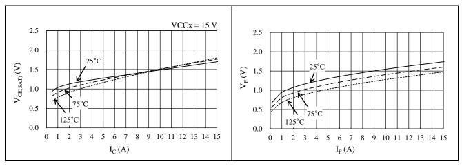
Figure 15-29. IGBT V<sub>CE(SAT)</sub> vs. I<sub>C</sub>
