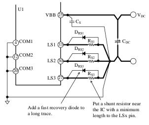
Figure 12-7. Connections to LSx Pin
