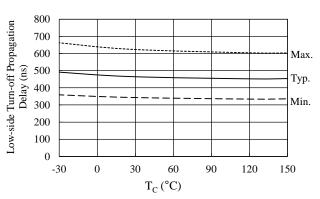
Figure 15-18. Low-side Turn-off Propagation Delay vs.  $T_C$  (from LINx to LOx)
