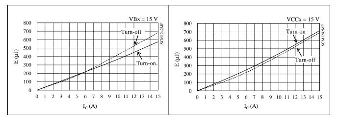
Figure 15-41. High-side Switching Loss ( $T_J = 125 \text{ °C}$ )
