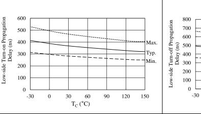
Figure 15-17. Low-side Turn-on Propagation Delay vs.  $T_C$  (from LINx to LOx)
