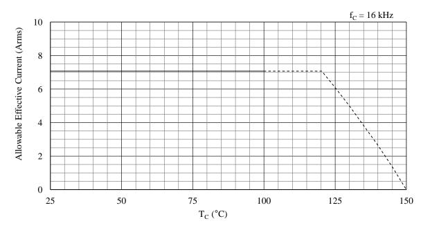
Figure 15-56. Allowable Effective Current ( $f_c = 16 \text{ kHz}$ ): 10 A Device
