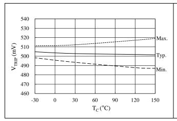
Figure 15-23. OCP Threshold Voltage,  $V_{TRIP}$  vs.  $T_C$
