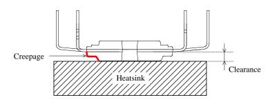
Figure 5-1. Insulation Distance Definitions
