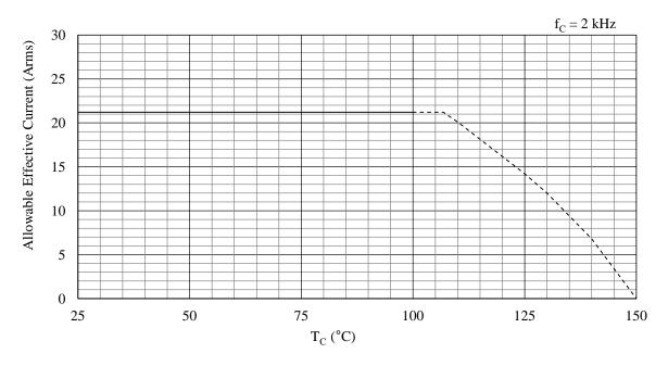
Figure 15-61. Allowable Effective Current ( $f_c = 2 \text{ kHz}$ ): 30 A Devices
