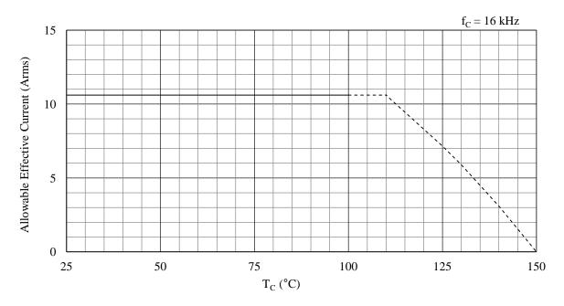
Figure 15-58. Allowable Effective Current ( $f_C = 16 \text{ kHz}$ ): 15 A Devices
