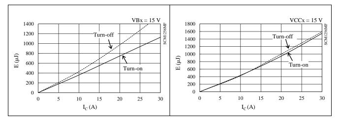
Figure 15-53. High-side Switching Loss ( $T_J = 125 \text{ °C}$ )
