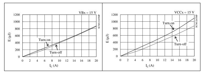
Figure 15-49. High-side Switching Loss ( $T_J = 125 \text{ °C}$ )
