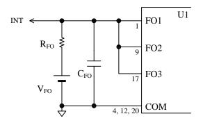
Figure 12-12. All-phase Shutdown Circuit
