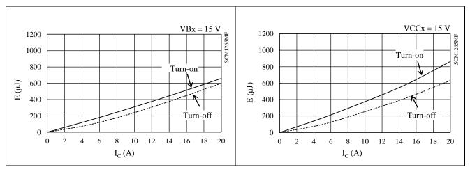
Figure 15-47 High-side Switching Loss ( $T_J = 25 \text{ °C}$ )
