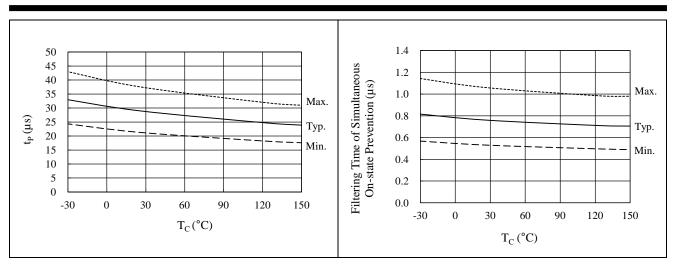
Figure 15-25. OCP Hold Time,  $t_P$  vs.  $T_C$
