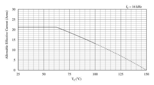
Figure 15-62. Allowable Effective Current ( $f_C = 16$  kHz): 30 A Devices
